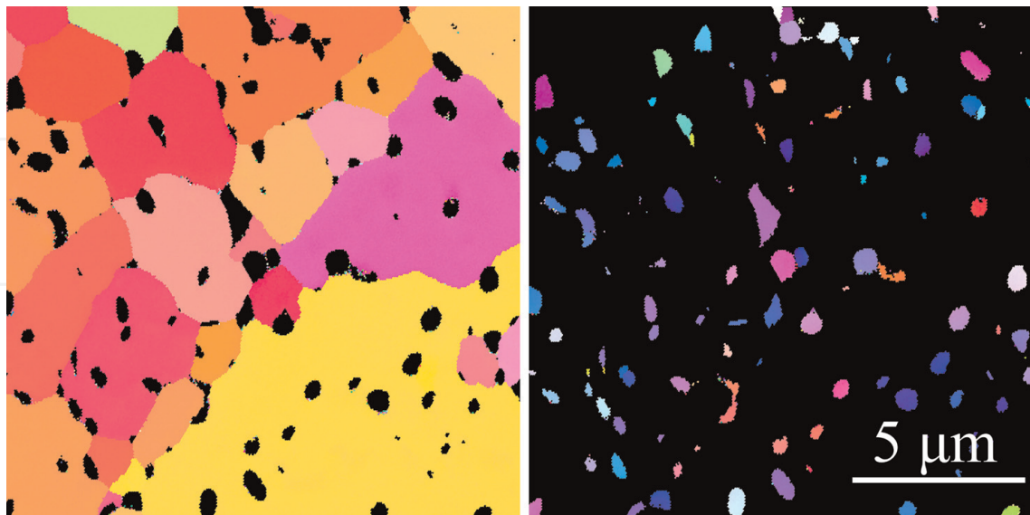
Figure 3 Example of EBSD analysis of precipitates: bcc Zr precipitates containing Nb and hcp Zr matrix in a Zr-2.5Nb alloy [2].
